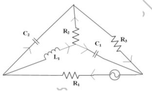
**40.** Draw the graph of the network shown in figure. Select a tree and write i. Incidence Matrix ii. Tie set matrix iii. Cut-set Matrix
